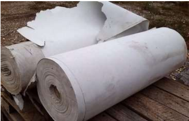
Asbestos duct insulation
