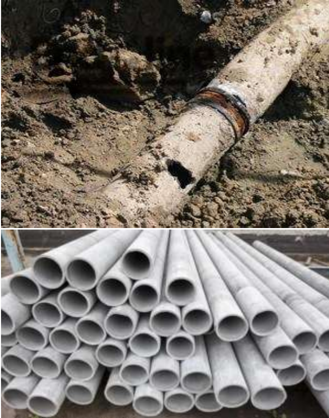
Asbestos-cement pipes for water supply systems
