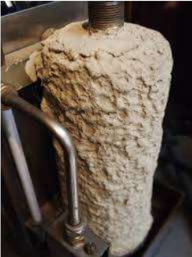
Thermal insulation of old gas water heaters
